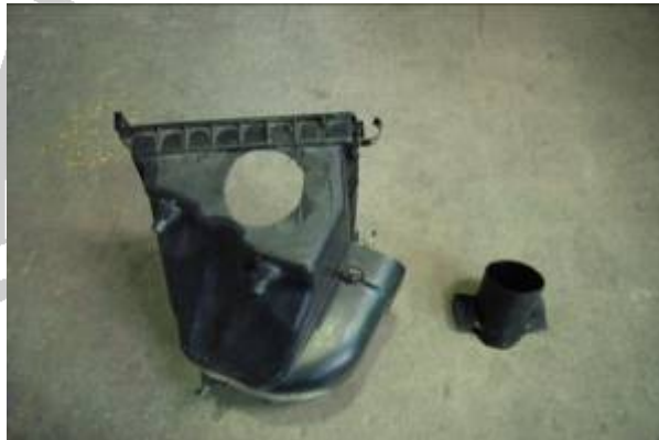
3.30 To prepare the air box, place the template over the air box using the trim line as a guide
