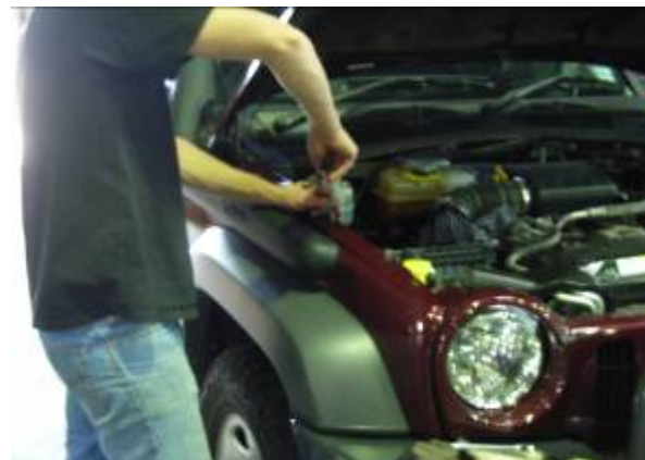
3.53 Re-install all the panel bolts and the wheel arch guard
