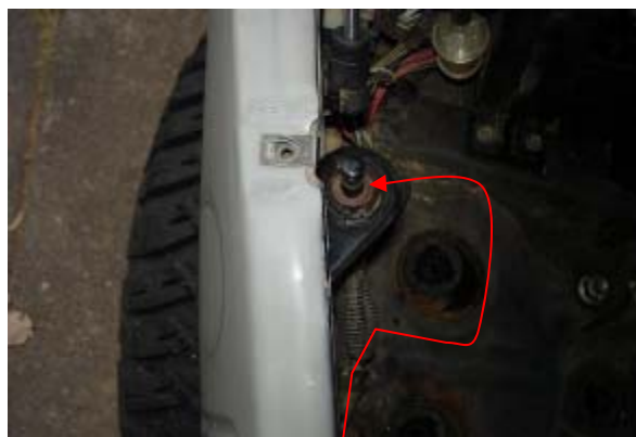
3.19 On the LTD models, there is a 'Bonnet Alarm' pin located on the inner guard.
