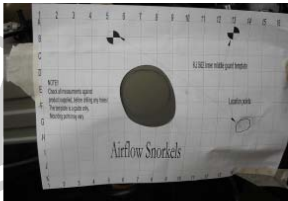
3.22 Cut the hole as marked
