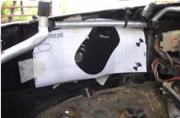
3.27 Using the inner template, line up the reference points
