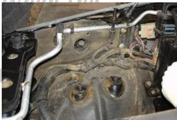
3.20 Remove the air box
