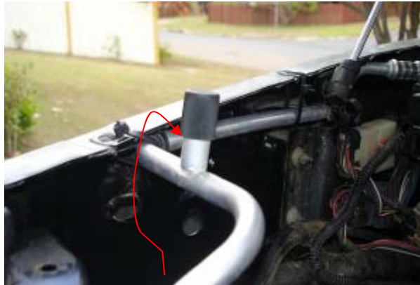
3.26 Unclip the air condition pipe and the wiring harness to allow easy access when cutting the hole in the inner guard
