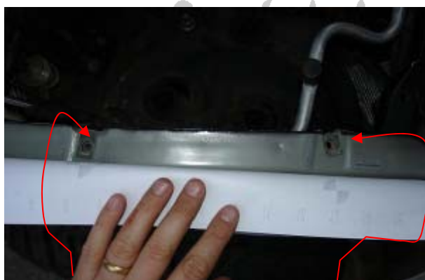
3.23 Use the inner middle guard template to line up of these points
