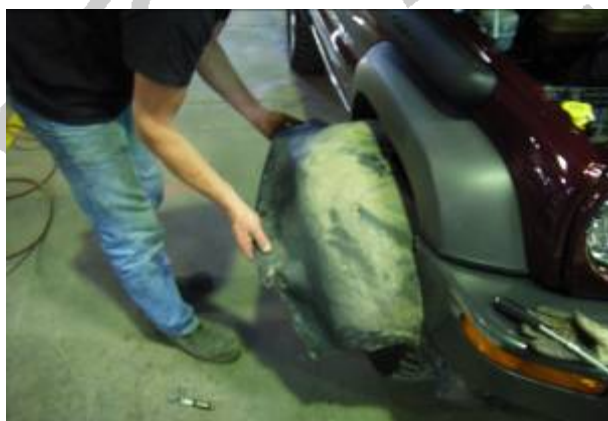
3.54 Refit the mud splash panel
