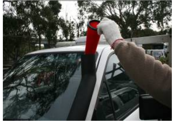
4.2 Install Pre-cleaner filter sock SP065B
