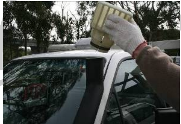
4.4 Re-install the Air ram SP063
