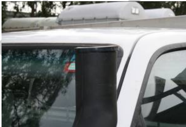
4.3 Air sock should neatly fit into the top of the snorkel body
