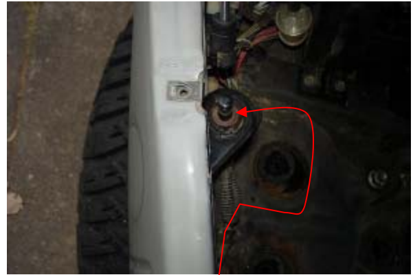
3.19 On the LTD models, there is a 'Bonnet Alarm' pin located on the inner guard.
