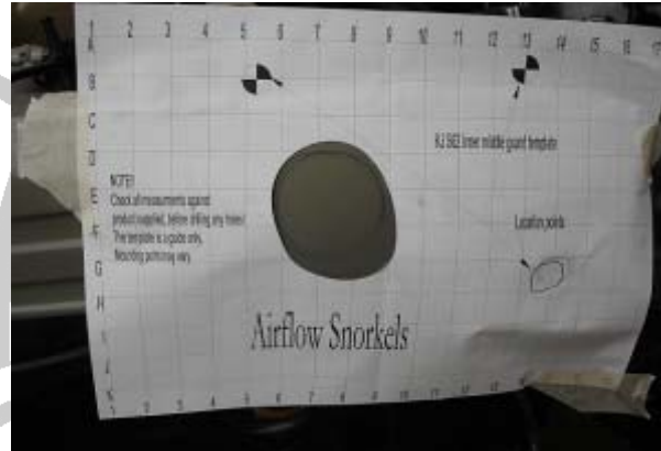
3.22 Cut the hole as marked
